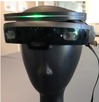
Figure 1: Modified HoloLens device with external LED display.
